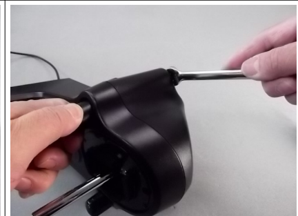
Remove Clamp screw
